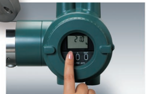
Infrared switches enable operation without opening the display cover
