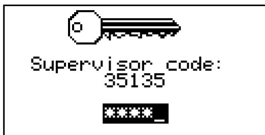
Afterwards, a number with five digits is displayed, and the company DIGITRONIC has the specific supervisor number for this number. (The number is shown on the display until the voltage supply is shut off
